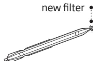
Remove the tool from the packaging. The tool has two ends, one for removal and one with the new O-Cap filter.
