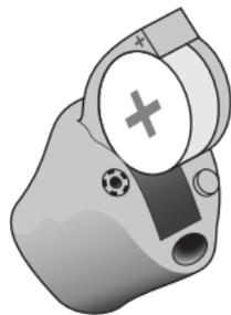
Insert the new battery into the battery drawer. Make sure the + side faces the + on the battery drawer.
