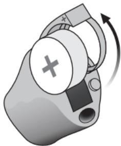
Fully open the battery drawer. Remove the battery.
