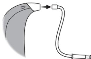
Pull the thin tube out of the hearing aid.
