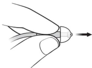
Hold on to the end of the thin tube and then pull off the dome.
