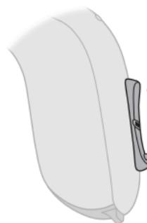
Apply a very long press (4 seconds) to either end of the button to mute the hearing aid. To reactivate the hearing aid, push the button briefly.
