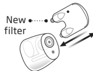
Push the empty pin into the wax filter in the MicroMold and pull it out.
