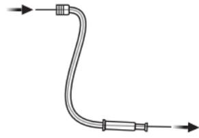
Push the cleaning tool all the way through the thin tube.
