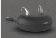
Oticon Opn S™ miniRITE R is a discreet style powered by rechargeable lithium-ion battery. The inductive charger ensures reliable and fast charging within 3 hours for a full charge.
