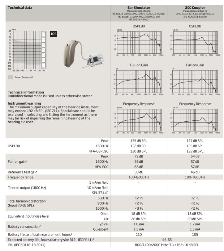
Measured with the gain control of the hearing aid set to its full-on position minus 20 dB and with an input SPL of 70 dB. This is to obtain a gain response equal to the full-on gain response from e.g. IEC 60118-0+A1:1994 but without influence of feedback.
