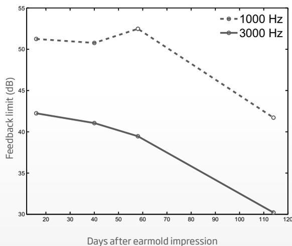
**Figure 3. Impact of the growing ear on the feedback limit as a function of time.** The feedback limits at 1000 Hz (dashed line) and 3000 Hz (solid line) are shown as a function of time for the left ear of a 16-month-old child. The feedback measurement was repeated during four visits over 110 days. A higher feedback limit allows more gain in the instrument.
