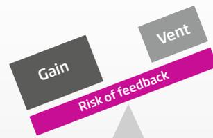
**Figure 4. The balance between vent and gain.** A correct balance between the amount of venting and gain in a fitting will keep the risk of feedback in check. The assumption is that both large venting and high gain are desirable. However if one goes up, the other most come down.
