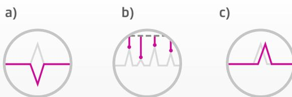
**Figure 5. The Oticon symbols illustrating the three core elements of the Inium feedback shield: a) Phase inversion - The use of destructive interference to cancel the feedback signal. b) Gain Control - The use of continuous feedback limit estimation to temporally limit the gain to eliminate feedback. c) Frequency shift - To introduce a shift in the frequency response to allow more frequent updates of the filter. In Sensei the frequency shift is only applied when it is called for.**
