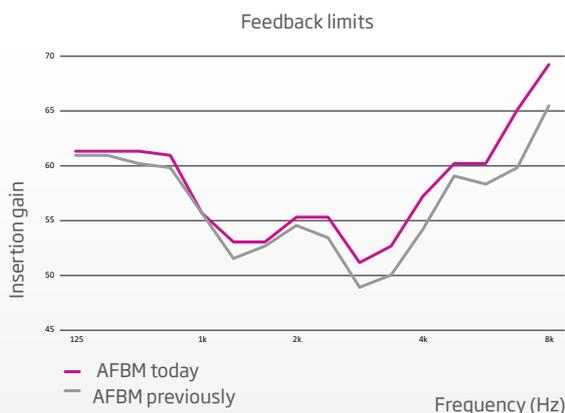
**Figure 7. Oticon's new anti-feedback system compared to the previous one.** Feedback limits are shown as a function of frequency. The magenta curve shows how the Automatic Feedback Manager (AFBM) sets the feedback limit with the Inium feedback shield, and the grey curve how it is set for Oticon's previous anti-feedback system.
