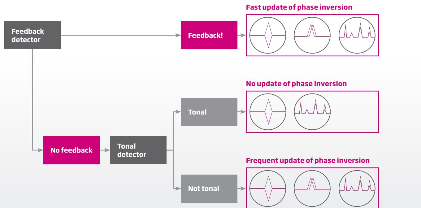
Figure 2. Schematic modes and detectors in feedback shield.
