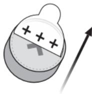
Remove the sticky label from the + side of the new battery.
