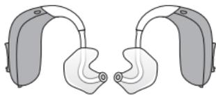
Make sure you are able to identify which mold is for which instrument before disconnecting them from the instruments.
