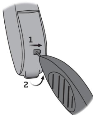
Insert the tip of the tool into the small hole at the back of the battery drawer.
