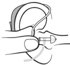
Hold the bend of the tube between your thumb and index finger. The ear piece should point towards the ear canal opening.
