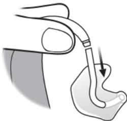
Disconnect the tube and mold from the hook. Hold the hook firmly, when pulling off the tube. Otherwise the instrument may be damaged.
