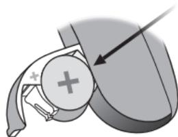
Insert the new battery into the battery drawer. Insert it from above, NOT from the side. Make sure the + side faces up.
