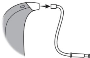
Pull the thin tube out of the hearing instrument
