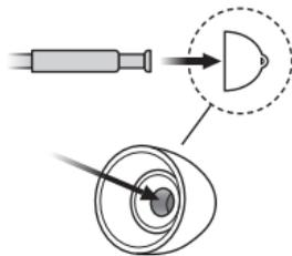
Place the thin tube exactly in the middle of the dome.
