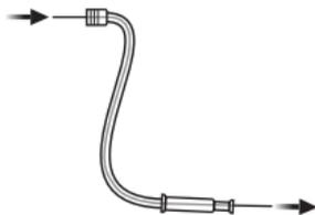
Push the cleaning tool all the way through the thin tube.
