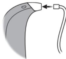
Reconnect the thin tube to the hearing instrument.
