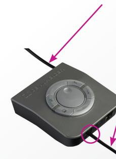
Connect the interface cable to the UI770 headset port.
