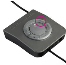
Ensure the headset/handset button on the UI770 box is deselected (not pressed down).
